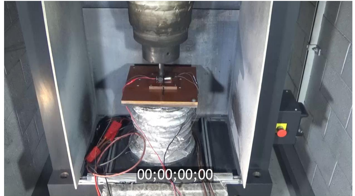
Post Overcharge Crush
